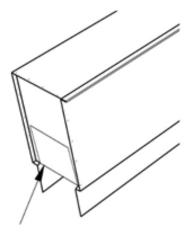
FOR CONTINUOUS OR SHORT END CAP APPLICATIONS, SHARPLY BEND THE AIR GATE UP AND AGAINST THE TOP SECTION. THIS RESULTS IN 2 1/2" OF FREE SPACE FOR THE DIFFUSER TO PASS THROUGH
